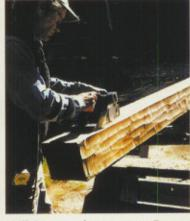
Will Beemer, above, uses a German power plane fitted with a curved blade to produce a convincing rough-hewn look. With the same tool, Anthony Zaya of Lancaster County Timber Frames power-planed an antique look onto the trusses of a new house in Westchester County, New York, right, "It would have taken 10 guys a whole week to do them by hand," says Zaya. "We were done with each set in about three hours."
